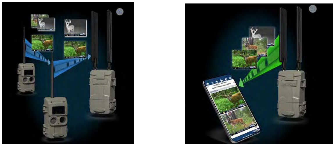
Figure 1. Cuddelink Camera system – Up to 10 cameras send images via ‘daisy chain’ link to ‘home’ camera, the cell ‘home’ camera delivers images from all Cuddelink cameras to user via LTE.
